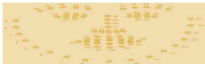
Figure. 22. Sixty Eight different landmarks of a face
