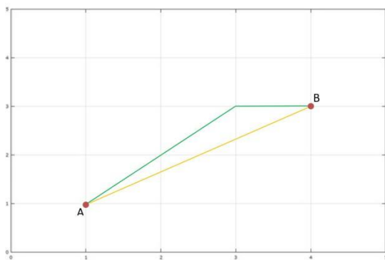
Figure 3: Trajectory from point A to B using paths in the form of lines corresponding to the Chinese checker metric.
