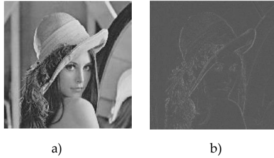
Fig. 3.7.1.3 (I): Applying the Neutrosophic Internal Boundary: a) Original Image b) Neutrosophic Internal Boundary Filtered Image
