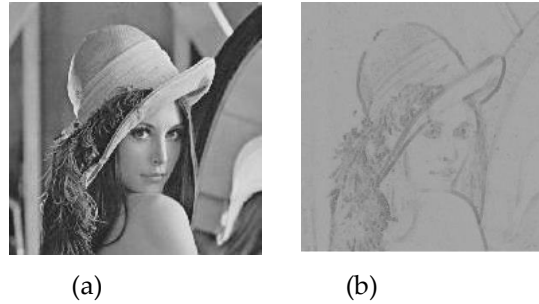
Fig.3.7.1.3 (II): Applying the Neutrosophic Internal Boundary: a) Original Image b) Neutrosophic Internal Boundary Filtered Image
