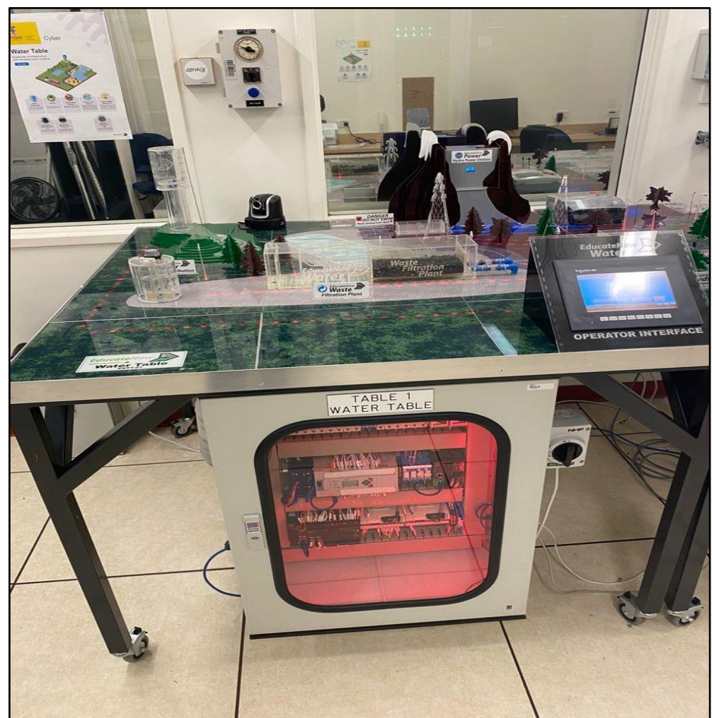
Figure 3. Water CPS testbed used at the IoT lab of UNSW Canberra.
