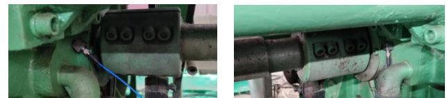
FIGURE 6. The journals and sensors at both ends of the loom spindle
